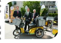
As a key part of its sustainability programme Austrian Post has now deployed seven Kyburz DXP electric tricycles following pilot tests. The tricycles have a 120kg load capacity with potential for an extra 150kg of load space on a trailer. They have a range of up to 100km and a top speed of 45km/h.
