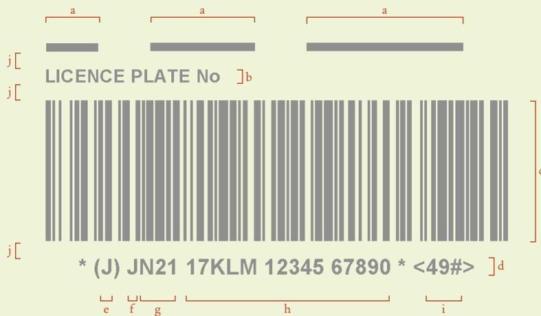
AN EXAMPLE OF HOW A PARCEL LICENCE PLATE IS CONSTRUCTED ACCORDING TO UPU STANDARD S26
