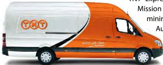
The Volkswagen Crafter 50 vans have sleeper cabs, GPS tracking and satellite phones. They will pick up and deliver urgent packages at mine sites, accommodating cartons, pallets and crates weighing up to 1,300kg.
