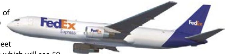
The wide-body 767 has a gross payload of 127,100 pounds and a flight range of 2,922 nautical miles. FedEx said the freighters would be approximately 30% more fuel efficient and have 20% lower operating costs than the MD10. It is projecting a 30% reduction in unit carbon emissions by 2020 across its fleet.
