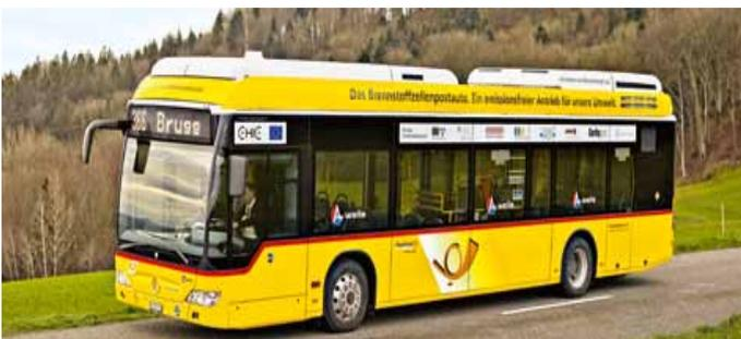
PostBus claims to be the first public transport company in Switzerland to use hydrogen fuel. The hydrogen will be generated by renewable sources. The company is also building a hydrogen fuelling station, initially for PostBuses but with a view to being made available to other vehicles as well.
