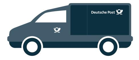
payload and 4m<sup>3</sup> of load space. It has battery capacity of 15kWh (100% from renewable energies), 130Nm torque, 30kW power (max. 45kW peak power), a maximum speed of 85km/h and a range of 120km.
